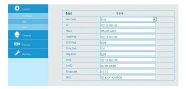
In this interface we can set the internet attribute of device, IP address, subnet mask, gateway and preferred domain server included. Make the internet configuration according to the actual situation.
