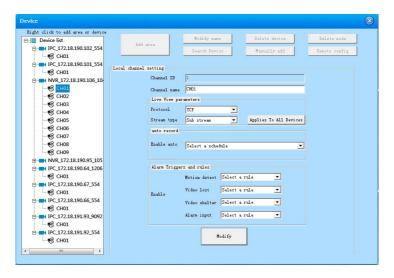
You can modify the parameters like Device Name, Port No., and User Name/Password etc. The default port No. is 554, and the default http port No. is 80.
